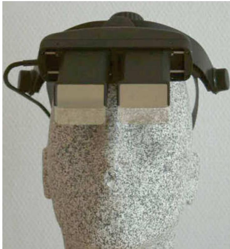
The LCD29-HMD is a specialized product designed for Augmented Reality applications. It is an optic-see-through device that projects an image or a streaming video through the near-the-eye micro-displays. The frameless design allows nearly unblocked vision.
