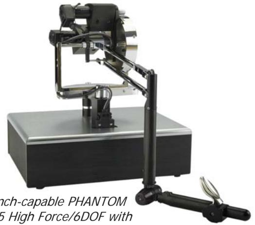
*Pinch-capable PHANTOM 1.5 High Force/6DOF with thumb-pad end effector
