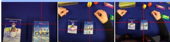
**36 Degree Lens    60 Degree Lens    96 Degree Lens (Standard)**
